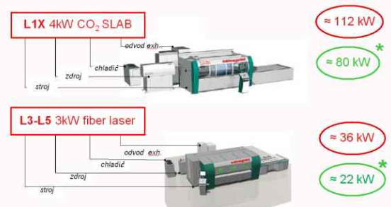
Spotreba energie 3kW Fiber vs 4kW CO 2
